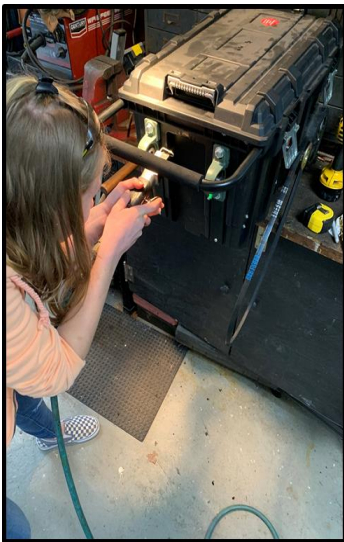
Figure 12: Using an air-saw, I am cutting a rectangle to insert the switch panel.
