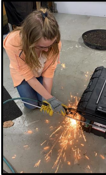
Figure 10: Using a cut-off tool, I am cutting the shaft to length.
