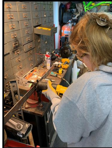
Figure 5: I am cutting metal braces from flat stock to reinforce box.
