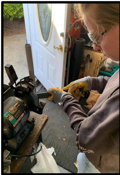
Figure 6: Using Bench grinder, I am smoothing the sides of the metal brace.
