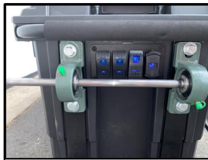
Figure 16: Switch Panel. The two left-most switches operate the lights, while the right switch controls the main power.
