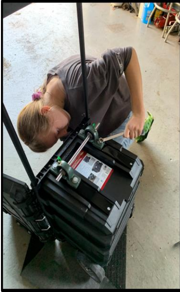
Figure 9: I am securing bearings onto metal braces with a wrench.
