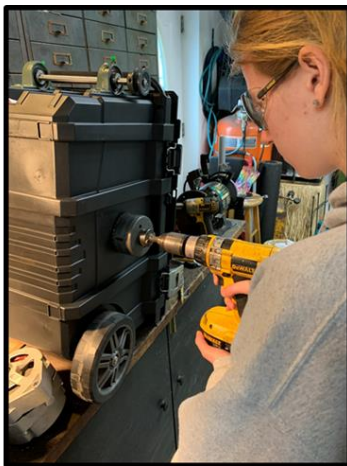
Figure 1: I am drilling main hole for alternator with a hole saw.
